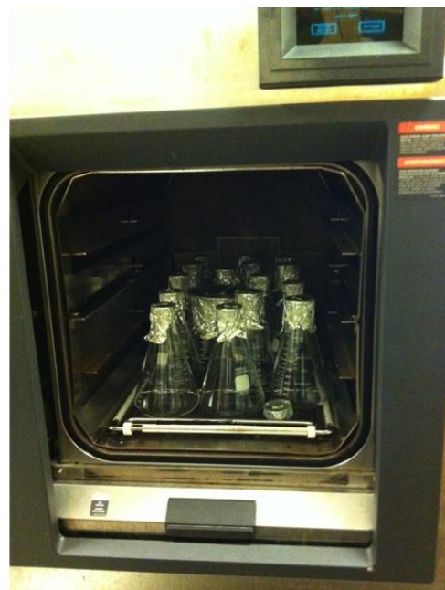
Figure 3. Autoclave for sterilization of seawater and glassware.
