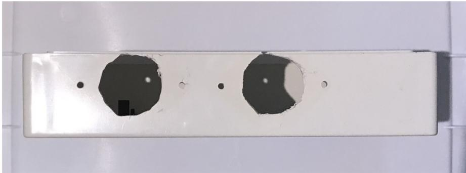
Drill a hole on the side panel for the barrel jack connector that will be used to plug in the power adapter.
