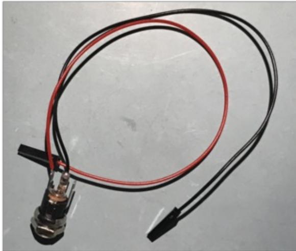
Strip and trim one end of two female jumper wires. Solder them with the barrel jack. We'll use this to connect the power adapter with the rest of the circuit.
