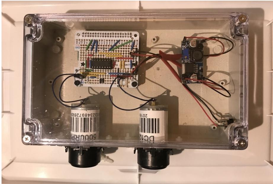
The heart of the dosing systems are peristaltic pumps, which reef-pi uses to pour liquid at fixed interval in a fixed speed.
