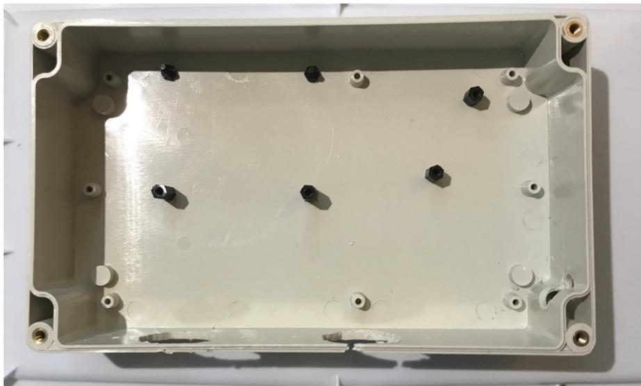
Once standoffs are fixed, mount the LM2596 module and the Raspberry Pi Zero
