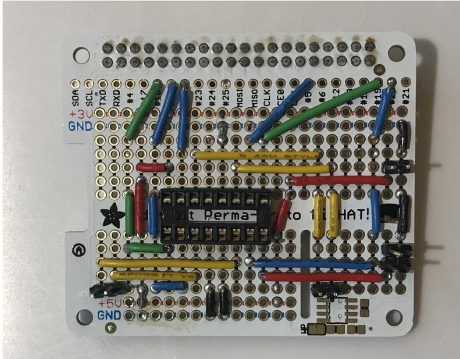
That's all, insert the L293D IC and we are good to go for mounting the circuit inside the enclosure and test it out.
