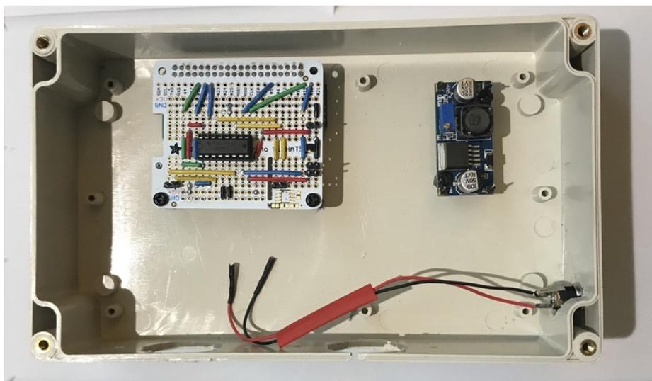
Once all the electronic components are mounted, attach the peristaltic pumps at last, and connect all the wires. Notice we are using the perma proto hat to create a small 12 V rail (on the right side) from which the LM2596 and the L293D (Vmotor) draw their power.
