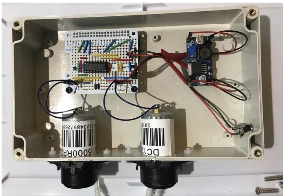
That's it, once all the components are wired, attach the clear case top and our dosing controller is ready for some testing and calibration
