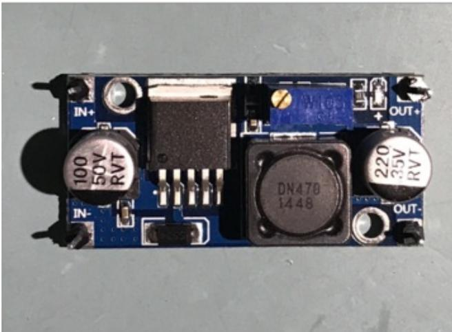
Solder male header pins on LM2596 module. We'll connect this with 12V rails on the perma proto board using female-female jumper pins
