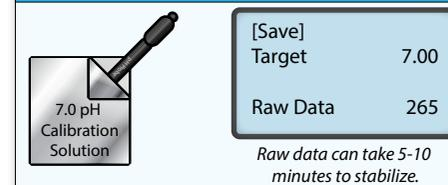
Once the raw data has stabilized, press [Enter] on [Save]. Calibration is complete. Rinse the probe in RO water. The probe is now ready for use.
