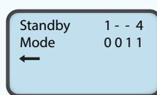
In this example, the channel will respond to Standby 1 & 4. It will: Turn off for Standby 1. Turn on for Standby 4. Ignore Standby 2 & 3.
