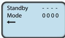
**Standby** sets which Standby modes will control the channel. The channel will ignore any Standby set with a dash (regardless of **Mode** Setting.)
