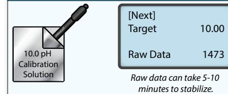
Once the raw data has stabilized, press [Enter] on [Next]. The target will change to 7.00. Rinse the probe in RO water. Place the probe in the 7 pH calibration solution.
