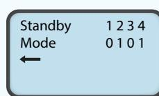
In this example, the channel will respond to all Standby modes. It will: Turn off for Standby 1 & 3. Turn on for Standby 2 & 4.
