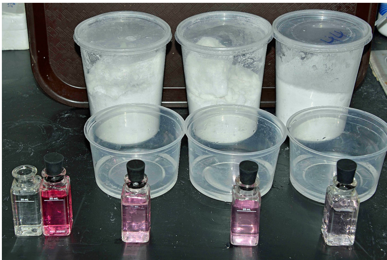
DPD chlorine test on three brands of sea salt – left to right; brands A, B, and C. Lighter pink color indicates less chlorine present after mixing. The dark pink vial on the left is the tap water control.
