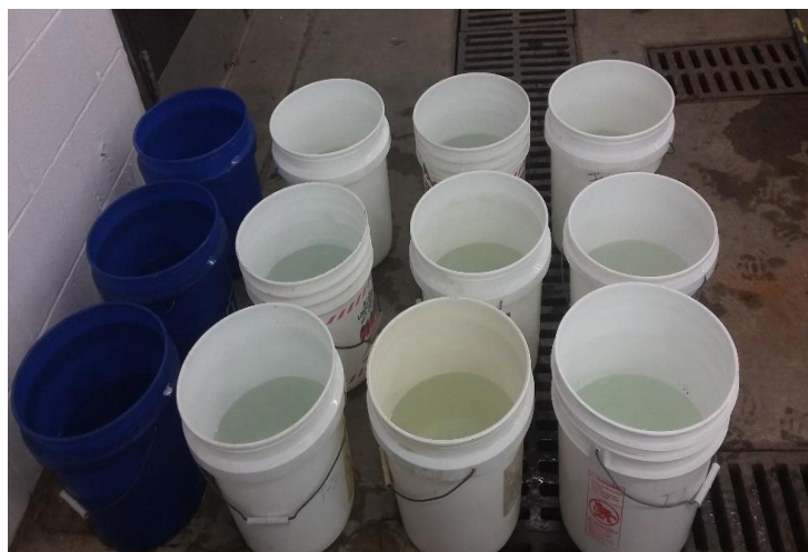
Fig 1: Treatment buckets (white) and Control buckets (blue) each with 10 liters of water
