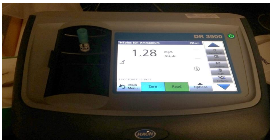
Fig 4: Using DR 3900 spectrophotometer by HACH® for reading concentration
