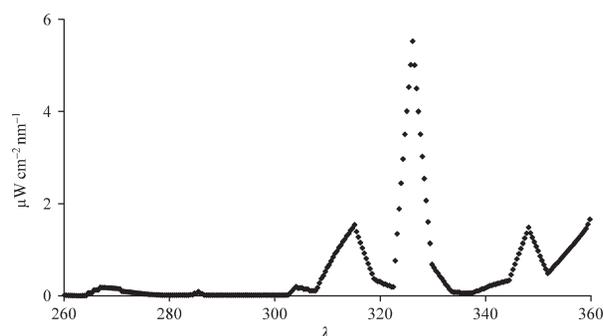
**Fig. 1.** Spectrum of UV light at a distance of 0.1 m from the light source.
